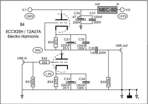
figure 4: MEC-50 in the MCML05 pre amplifier
