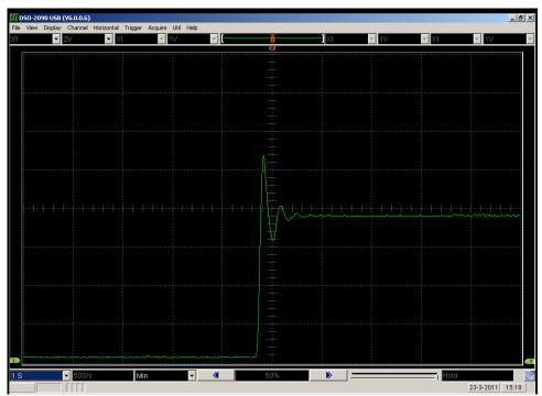
figure 5: time behavior MEC is not optimal tuned.
