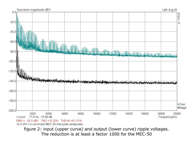
The MEC's are designed for so called C-L-C supplies and not for L-C supplies. Neither they are meant for transformer anode load applications.
