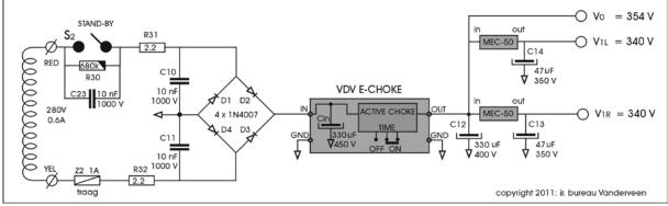
figure 3: E-choke and MEC in the UL40-S2 amplifier.
