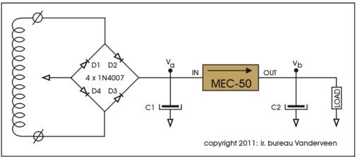
figure 1: connections on the MEC + current direction arrow
