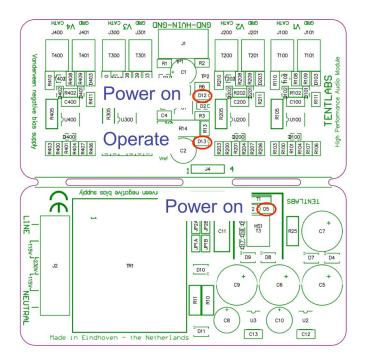
Both power on LEDs immediately light up after switch on
