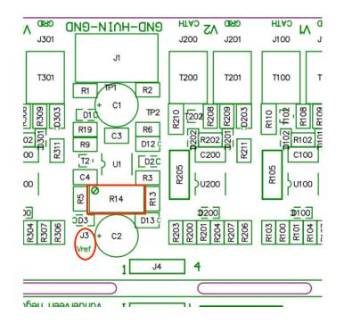
To decrease the bias current:Turn the trimmer counterclockwiseTo increase the bias current:Turn the trimmer clockwise
