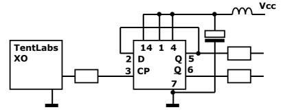
The flipflop gives a divide by 2 at both outputs Q and  $\underline{O}$ . Depending on the application, one of these can be taken (their phases differ 180 degrees)
