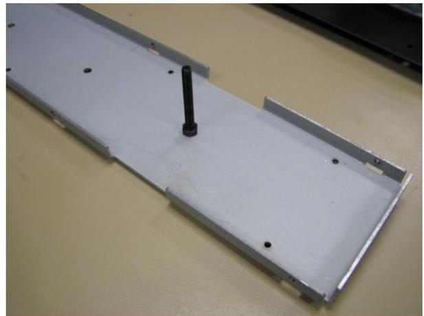
Take both wooden sides, place the metal sides on top of them (one orientation possible) and secure them using 6 screws from bag #1. Repeat this for the other side.
