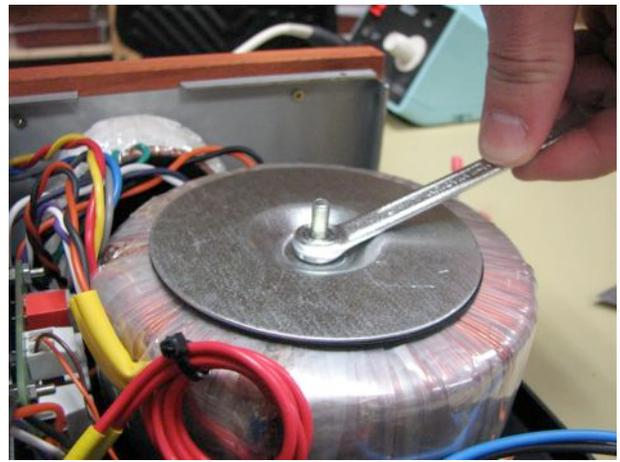
Take the remaining (unused) red wiring, cut the stripped ends and place 2 isolating sleeves on the ends. Take the tie rap and fit the wires as shown
