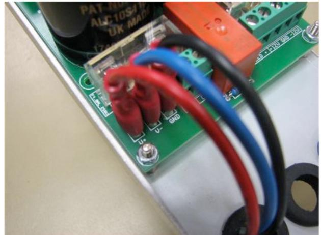
The other side of this wiring becomes connected to the UCD modules. Use the same color-coding:
