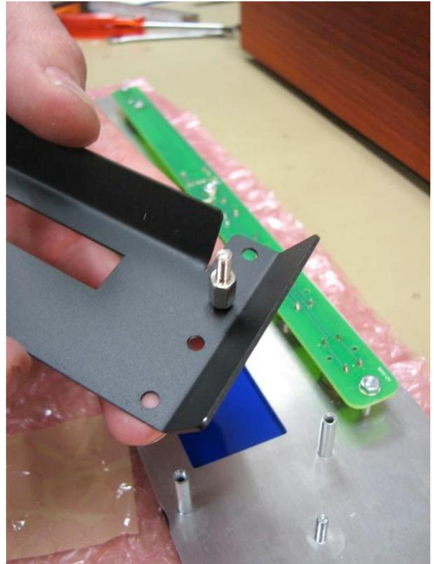
Place the front panel PC on the Display cover, and secure it with 4 M3 nuts.
